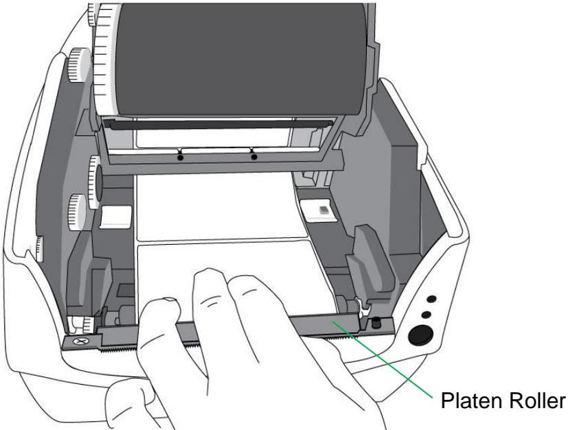
6. Press the lock of Media Guide at the right to adjust media guides' positions. Make sure media stays under the Media Shaft and centrally under both of the Media Guides.
