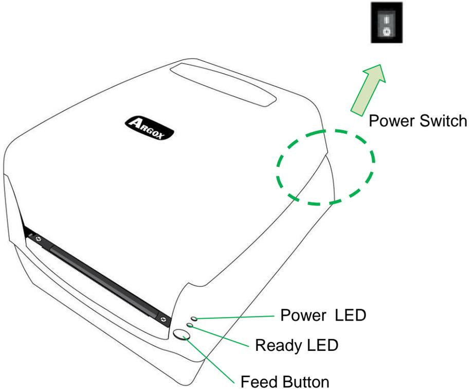
The following table explains printer controls and indicators' functions to help understanding LED indications and printer status:
