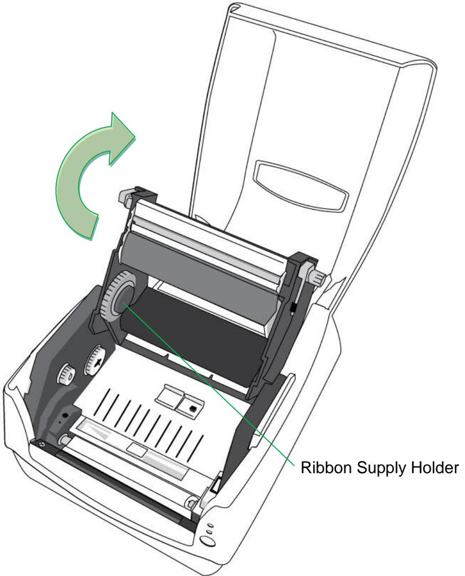
4. Install one ribbon roll and rotate it until the notches align and lock into the left side of Ribbon Supply hub, and then into the right.
