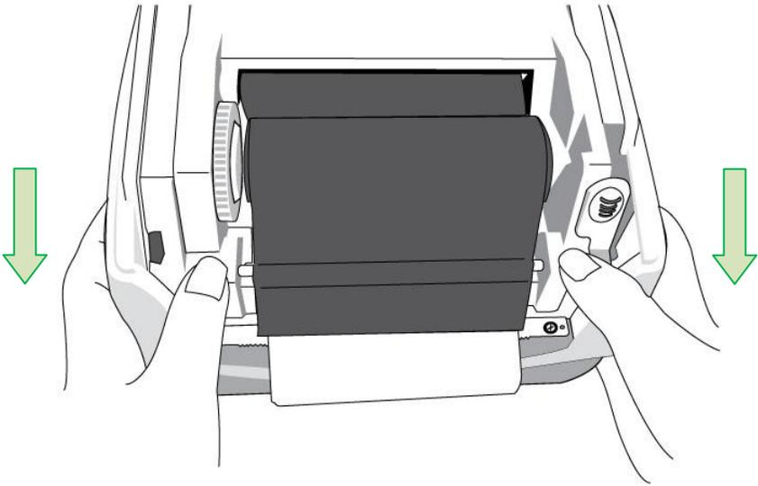
7. Rotate Thumb Wheel of Ribbon Pick-up Holder to remove slack and ribbon wrinkle, and to align the ribbon on the spindles.
