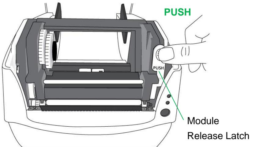
3. Lift up the printer module to check the Ribbon Supply Holder.
