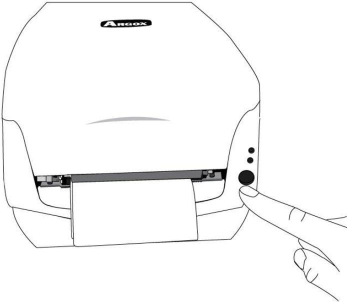
9. To tear media, pull the media edge against the Tear Bar as in the direction below:
