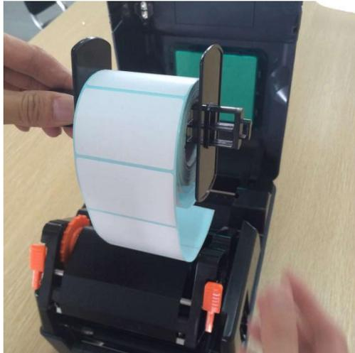
4. Press the printing head switch to open the printing head
