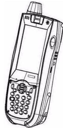
To reduce TCO, the PA968II is sealed to meet IP65 standards and has undergone multiple drop tests to prevent downtime.
