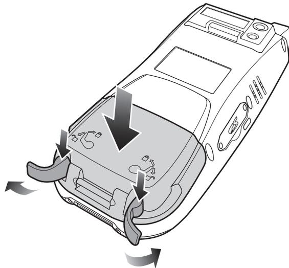
**NOTE:** Make sure the battery compartment cover is securely closed, or you may be unable to turn the terminal on.
