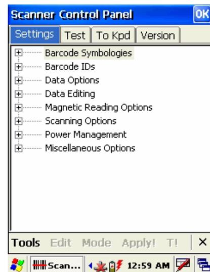
In the Scanner Control Panel screen, you can configure barcode scanner parameters such as enabling or disabling barcode symbologies, setting data transmission options, configuring magnetic and proximity reading options, and setting power management options. See *Barcode Symbologies* on page 36.
