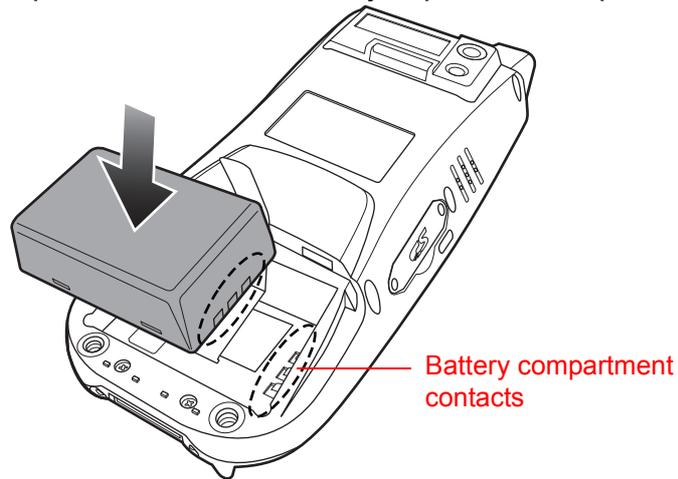
4. Slide the battery pack while simultaneously pulling the plastic tab until the battery clicks into place.
