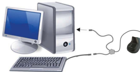
Figure 13. Connecting to the Host with Keyboard Wedge.
