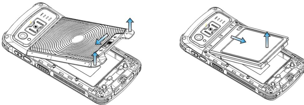
Step 1: Hold down the Power key for 5 seconds and then tap “Power off” to turn off the terminal. Slide the battery cover latch to the unlock position and remove the cover.
