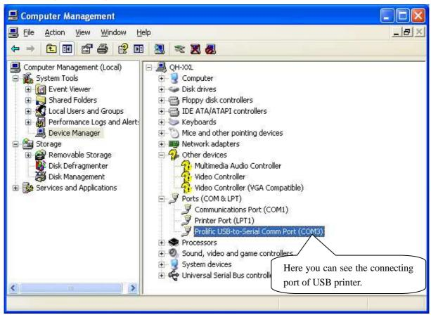
The connecting port of serial printer
