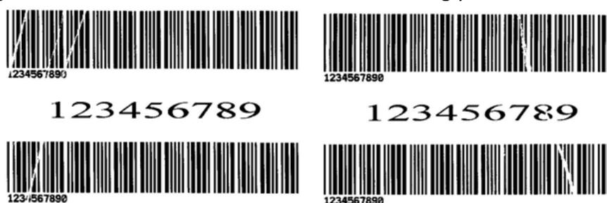
Once the printouts as above appear, the possible cause may be the unequal positions of Ribbon Bracket, which needs to be adjusted properly to make its heights equally the same at both sides. Steps to adjust are as below:
