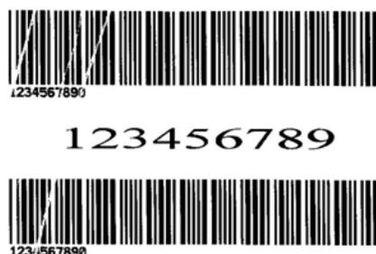
If the test print appears as Figure B, remain the screw at the left of Ribbon Bracket fixed, and then loose the screw at the right, and gradually fine-tune upward, until the print quality gets improved.
