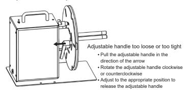
■ Core size adjustment and paper core installation or unloading
