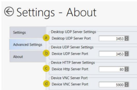
The 'Desktop UDP Server Port' (a) and 'Device UDP Server Port' (b) fields must be set to the same value as the matching ports on the remote device to ensure communication and remote configuration. The 'Device HTTP Server Port' (c) field must be set to the same value as the matching ports on the remote device to ensure communication and remote configuration. The 'Device VNC Server Port' field must be set to the same value as the matching ports on the remote device to enable Remote Control.
