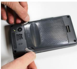
3. Grab the battery cover by the sides and lift it out of the way:
