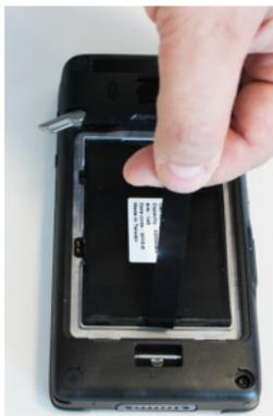
5. Insert the new battery pack into the slot (see [‘Install the Battery’](#) on page -9, steps 3 to 6).
