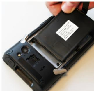
4. Insert the battery cover, bottom first, and press it into place:
