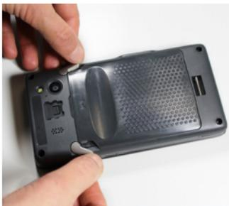
2. Grab the battery cover by the sides and lift it out of the way:
