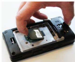
4. Slide the SIM card holder to the left to unlock it. Lift the holder:
