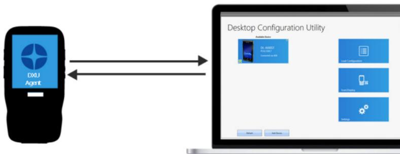
DXU configurations are stored as configuration files on the PC, and are transmitted to and from the DL-Axist as XML web pages. XML is a standard data format that is widely used for a variety of applications on the internet. Some data is encrypted in the XML file to protect your sensitive data from prying eyes, but most data which is not sensitive is transmitted in plain text that can be easily viewed and analyzed.
