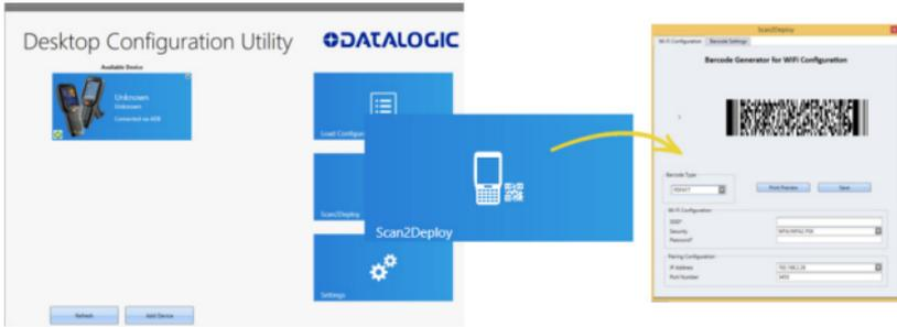
The **Scan2Deploy** button located on the main DXU page does not require an active connection to a device to create a 'Scan2Pair' barcode label. This button opens the Scan2Deploy dialog streamlined to create 'Scan2Pair' labels that can automatically connect a device to a Wi-Fi access point on your PC's subnet and to automatically connect it to DXU, adding it to DXU's '**Available Device**' list.
