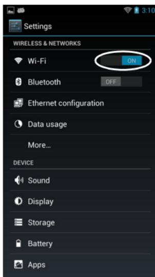
2. Tap **Wi-Fi**. The DL-Axist scans for available wi-fi networks within range and lists them. If the terminal previously connected to a wi-fi network, it automatically reconnects to the same network. Secured networks are indicated with a lock icon:
