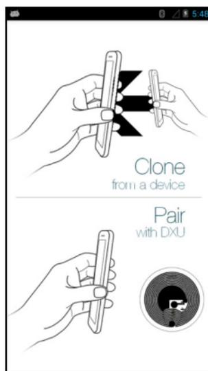
The cloning feature allows the settings of a device to be wirelessly cloned to another device within range.
