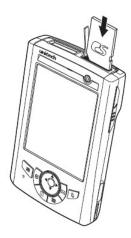
The card is secure when it is not protruding from the slot.
