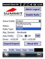
3. Under Status tab, you can see the IP address, signal strength and quality.
