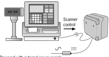
Powered with external power supply
