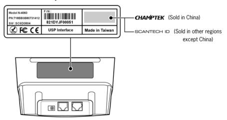
The scanner's serial number is found underneath the barcode label as depicted in the figure above. This official registration number is strictly related to the device. The supplier may ask for this number when the scanner needs servicing.
