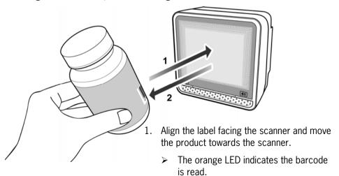
2. After the barcode is read, move the label from the scanner.
