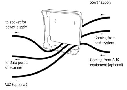
4. Make sure that connectors and cables are placed as indicated in the figure and attach the scanner to the bracket.
