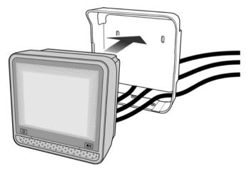
5. Plug the remote ends of all cables into the appropriate connections of your host POS-system.
